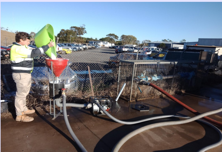
Pouring Polychlor Omega into the blending equipment hopper while filling the tanker from a hydrant
