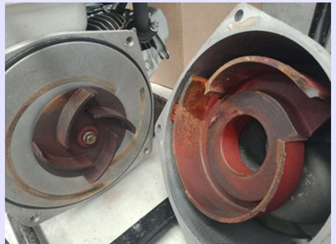
Inspection of the blending pump after pumping 1.4 tonnes of Polychlor Omega
